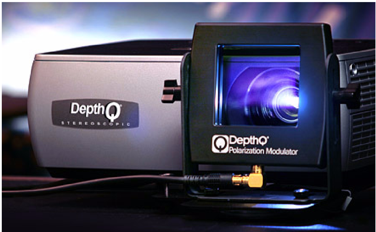
Figure 3: FPR-TN used together with high-speed projector and polarization-preserving projection-screen in order to generate 3D stereoscopic images using passive viewing-glasses.
